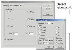
Specify the desired resolution and output paper size and orientation.
